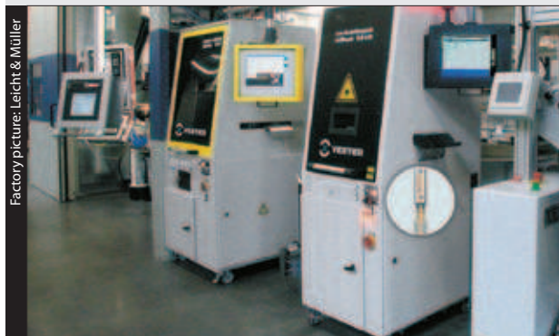
Stamping line with VVC 610 and LASERmark VLM 600 : Laser marking of continuously manufactured stampings
