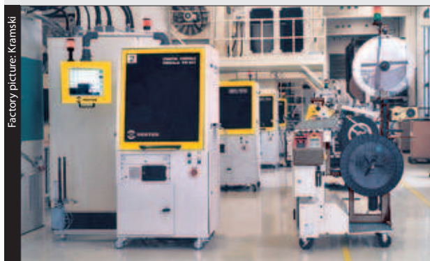
Test cell VVC 610 for stampings
